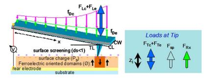
Fig. 1. Sketch of long range distributed loads, surface actuation, and tip loads acting on an integrated tip and cantilever during PFM.
