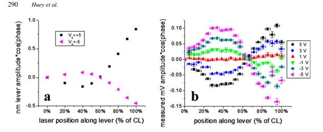
*Fig. 3.* Simulated (a) and experimental results (b) of the measured first harmonic response of a cantilever to periodic tip/lever biasing as a function of position along the lever and DC offset.
