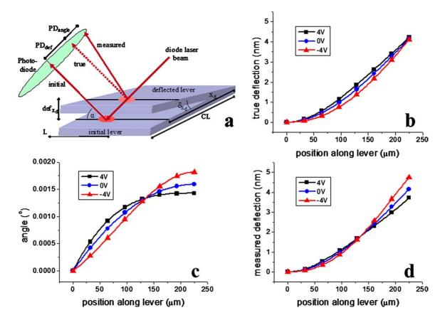
*Fig.* 2. Sketch of typical AFM sensitivity to angle (a), as well as the theoretical true deflection (b), angle (c), and measured deflection (d) along the lever.
